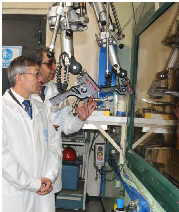
Mr. Dazhu Yang, IAEA Deputy Director General, Head of the Department of Technical Cooperation, observes the ININ hot cell for the production of radiopharmaceuticals. (Photo credit: ININ)
