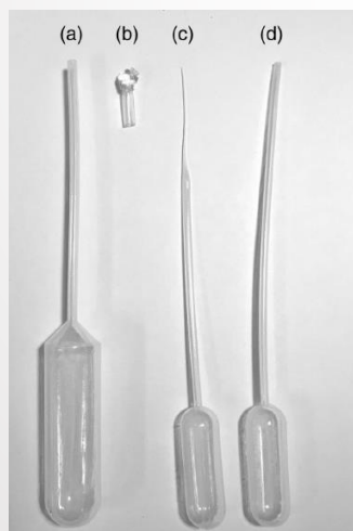
Fig. 2. (a) a 15.3 mL pipette, b (tubing cap), (c) modified tip of a (d) 4.5 pipette
