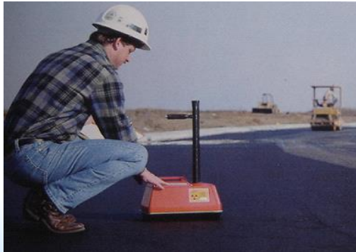
Mobile moisture/density gauge with Am-241/Be and Cs-137
