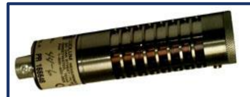
Side wall GM tubes
