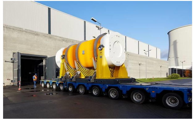
Test run of empty Castor® HAW28M cask at Biblis storage facility
