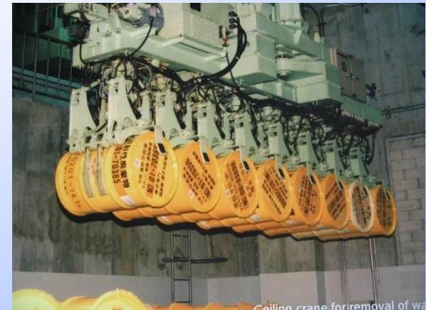
ceiling crane for removal of waste
