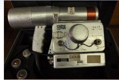
Scintillation survey meter designed for geological survey
