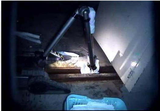
Wiping work with a robot
