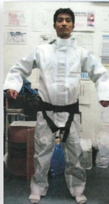
Protective suit made of Zylon
