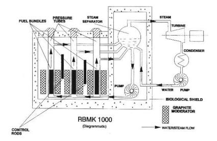
Operator actions triggered such excessive increase of power in the fuel that it most probably disintegrated in one part of the core. The first steam explosion moved 2000 tons reactor cover and then it was triggered combustion of the graphite moderator.
