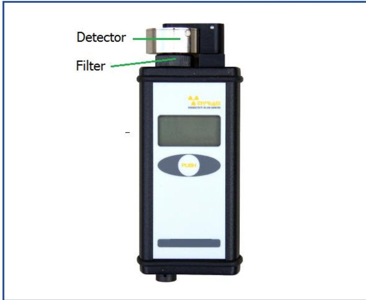
Portable planar silicon detectors for alpha spectrometry
