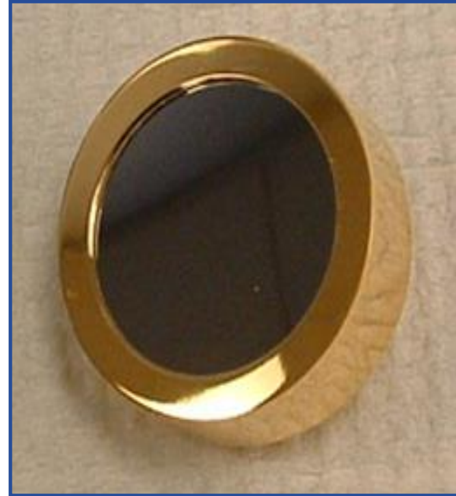
Typical PIPS detector
