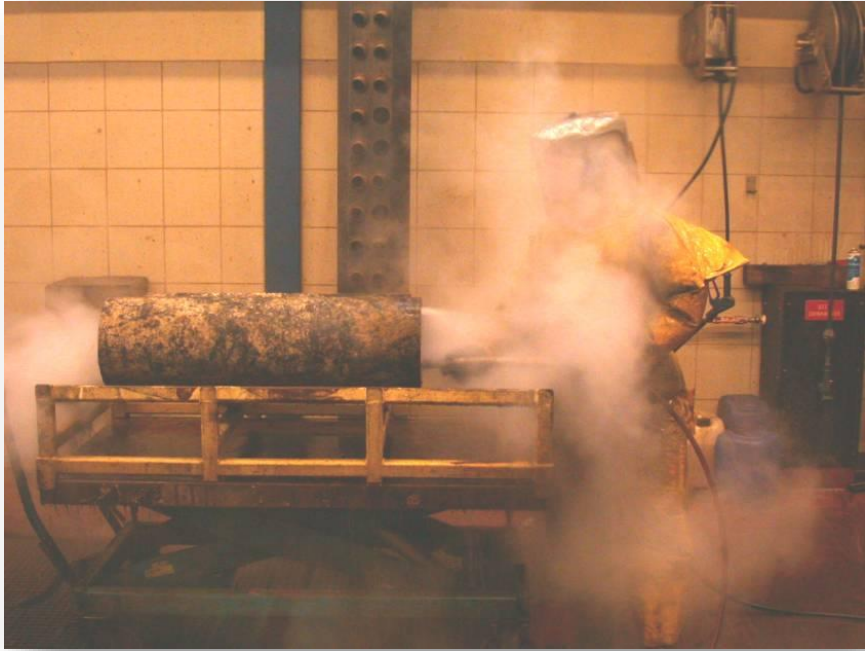
Scale removal using high pressure water jet
