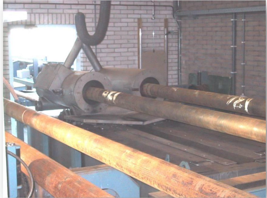
Dry drilling of tubulars with closed extractor system
