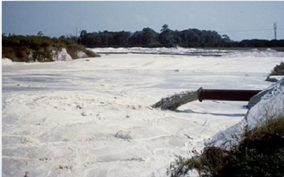
Phosphate rock tailings returned to the mined-out area
