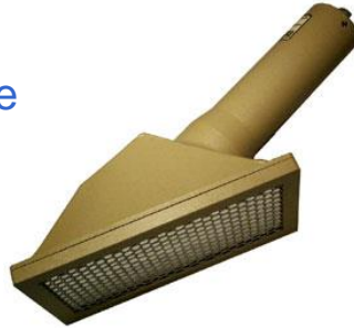
Beta probe Plastic scintillator
