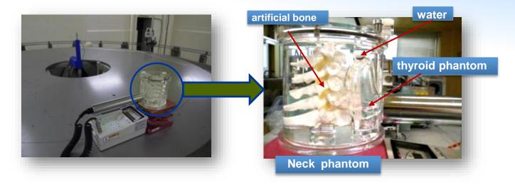
The <sup>133</sup>Ba solution with the same mass of the thyroid gland was put in the neck phantom.
