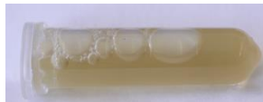
Figure 4. \sim 2 mL liquid after re-suspension and combination of 11 pellets (derived from 80% (\text{NH}_4)_2\text{SO}_4 precipitation)
