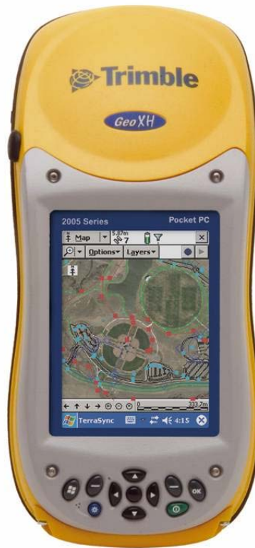
Figure 2. Trimble's "GeoXH" Windows CE GPS field computer.
