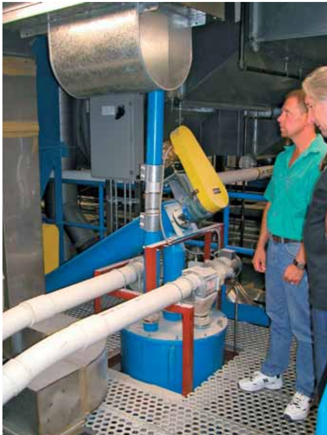
FIGURE 3 Augers, hopper and balance to deliver high-volume diet ingredients from storage room to cooking room and kettles below. (OKSIR facility, Osoyoos, Canada)
