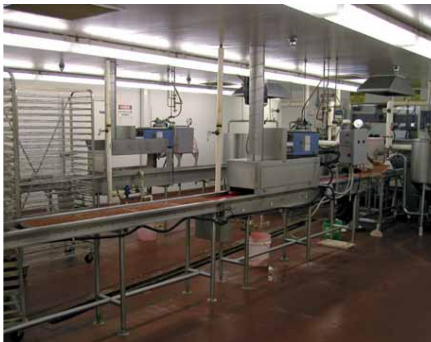
FIGURE 6 Two parallel diet-dispensing lines with belts showing enclosed aluminium portions (with blue units) that include paraffin wax sprayers and steam scarifiers. (OKSIR facility, Osoyoos, Canada)
