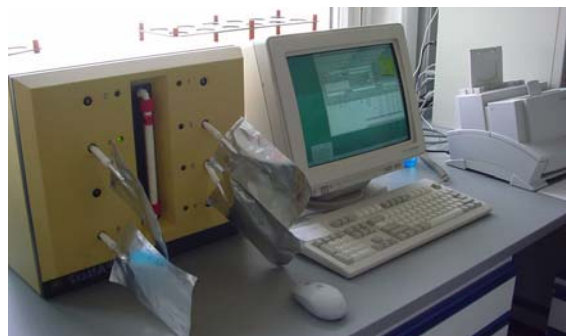
Figure 3. Laser based system for breath test analysis.
