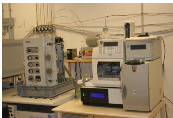
Figure 10. Schematic isotope ratio monitoring liquid chromatography mass spectrometer system (IRM-LC/MS).
