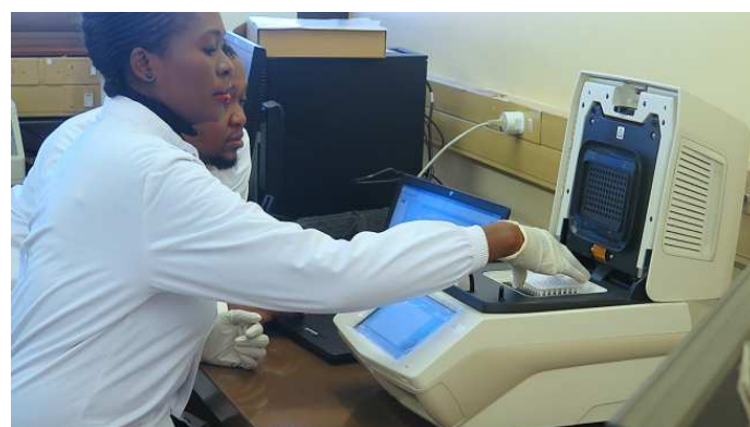
Scientists of the Animal Diseases Laboratory of BNVL using a real time PCR machine donated by the IAEA earlier this year to check blood samples from cattle for transboundary animal diseases. (Photo: M. Gaspar/IAEA).
