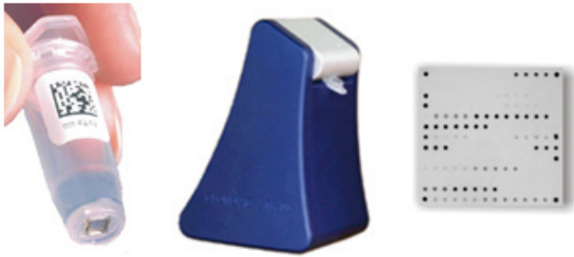
Figure 1. Clondiag Chip technologies ArrayTube (AT) platform. From left to right: array tube (with probe array chip on the bottom of the tube), the ATR 03 reader (connected to a PC or laptop to run image acquisition and analysis), magnification of probe array chip (detection reaction consists of horseradish peroxidase and HRP-substrate tetramethylbenzidine which reacts to form a blue precipitate).
