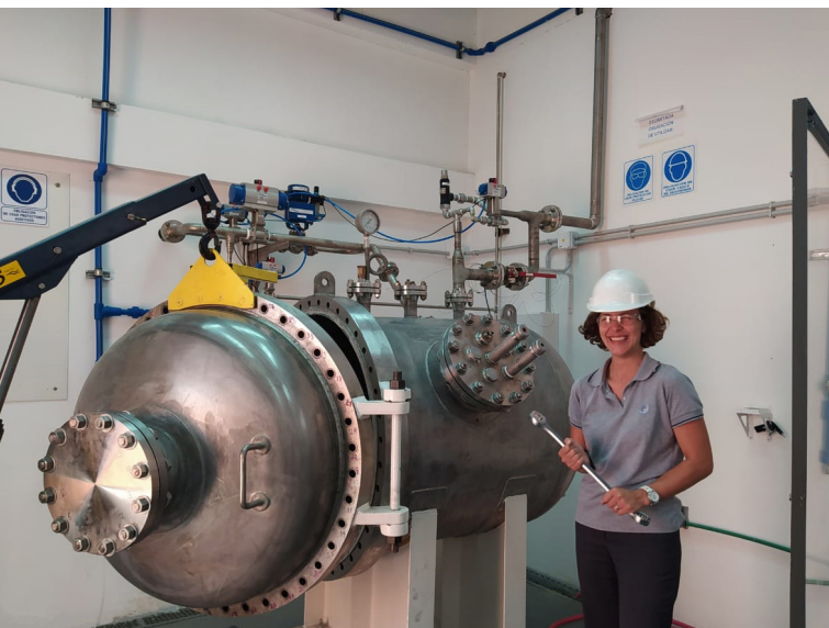
A 'loss of coolant accident' vessel used in reactor accident simulations. The IAEA supported a fellowship for a staff member from the nuclear research institute, ÚJV Řež, to the Argentinian National Atomic Energy Commission (CNEA) to build capacities to evaluate the environmental impact on electrical components in nuclear power plants. (Photo: Z. Sarsounova/ÚJV Řež)
