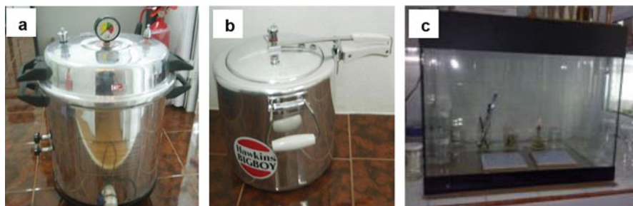
Fig. 10.5 (a) Stericlave. (b) Pressure cooker. (c) Low-cost, glass hood
