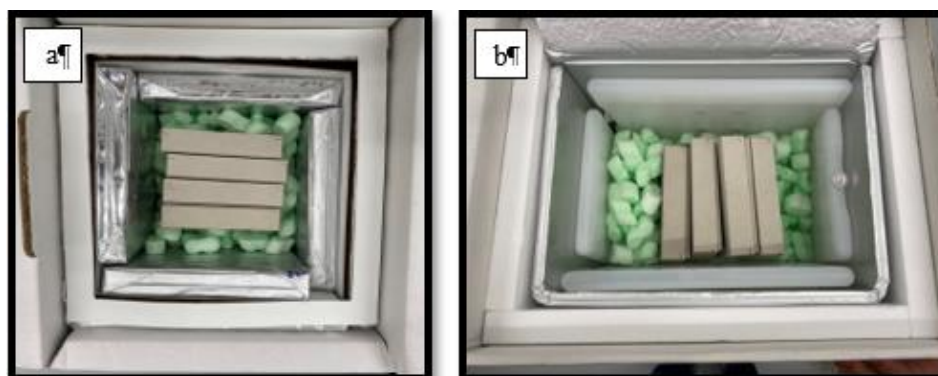
Figure 7. a) Inside view of a box used for chilled pupae shipment conditions, b) Inside view of a box used to ship pupae at ambient temperatures.
