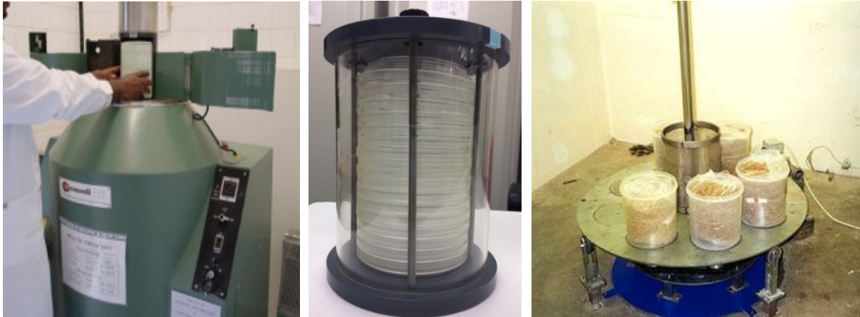
Figure 1. Examples of commonly used gamma-ray irradiators. A) Self-contained Gamma Cell 220 with an open sample chamber in the load position, B) a custom-made canister based on stacked petri dishes, and C) a panoramic irradiator where the source is lifted out of a dry pit during irradiation to the center of turntables with samples placed on top.
