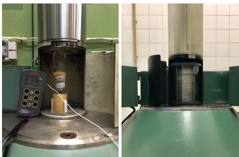
Figure 2. Examples of samples placed in the center of the chamber (in small cups, left, or in petri dishes, right). These are surrounded by a 4mm thick PMMA tube, which provides adequate build-up material. The temperature is taken before and after exposure. The temperature information is important for the dosimetry
