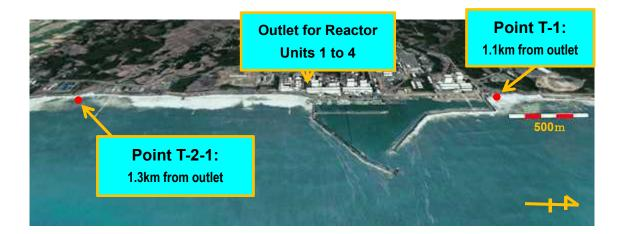
The concentrations of Cs-134 and Cs-137 monitored at the sampling points T-1 and T-2-1 from 10 December 2013 to 27 June 2015 are shown in the following figure. The values under the limit of detection are not plotted on the figure. Seawater samples are taken every day except for days of bad weather.
