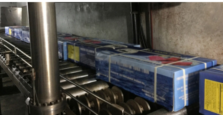
At the Research and Development Centre for Radiation Technology in Ho Chi Minh City a technique was introduced in 1999 with support from the IAEA and FAO, in which food products undergo an irradiation process to extend their shelf life and kill potentially harmful microorganisms. (Photo: E. Marais/IAEA)
