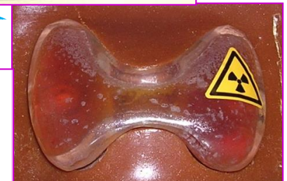
Livermore Thyroid Phantom, IRSN (France)
