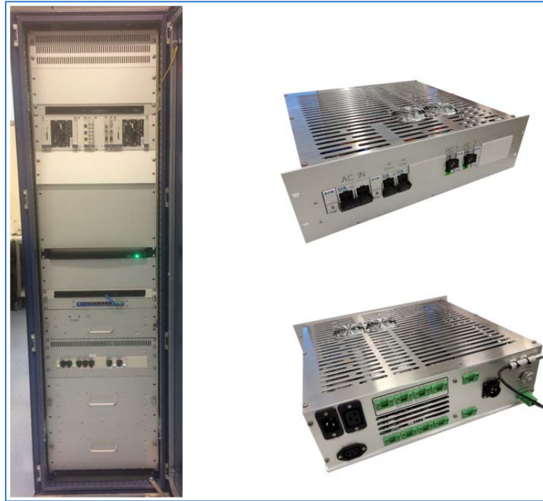
Figure 71: Typical UMS system operating on full DC power with its DC power management module
