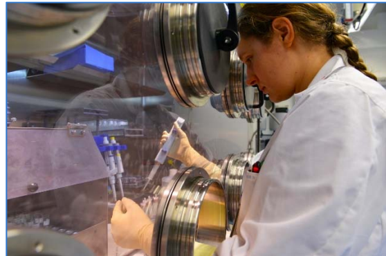
Figure 3: Aliquoting samples in the Pu Lab
