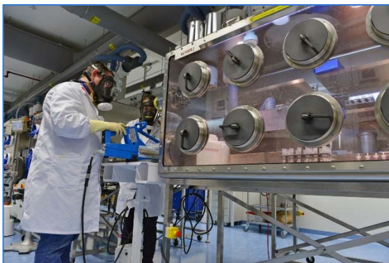
Figure 4: Bagging out samples in Pu Lab
