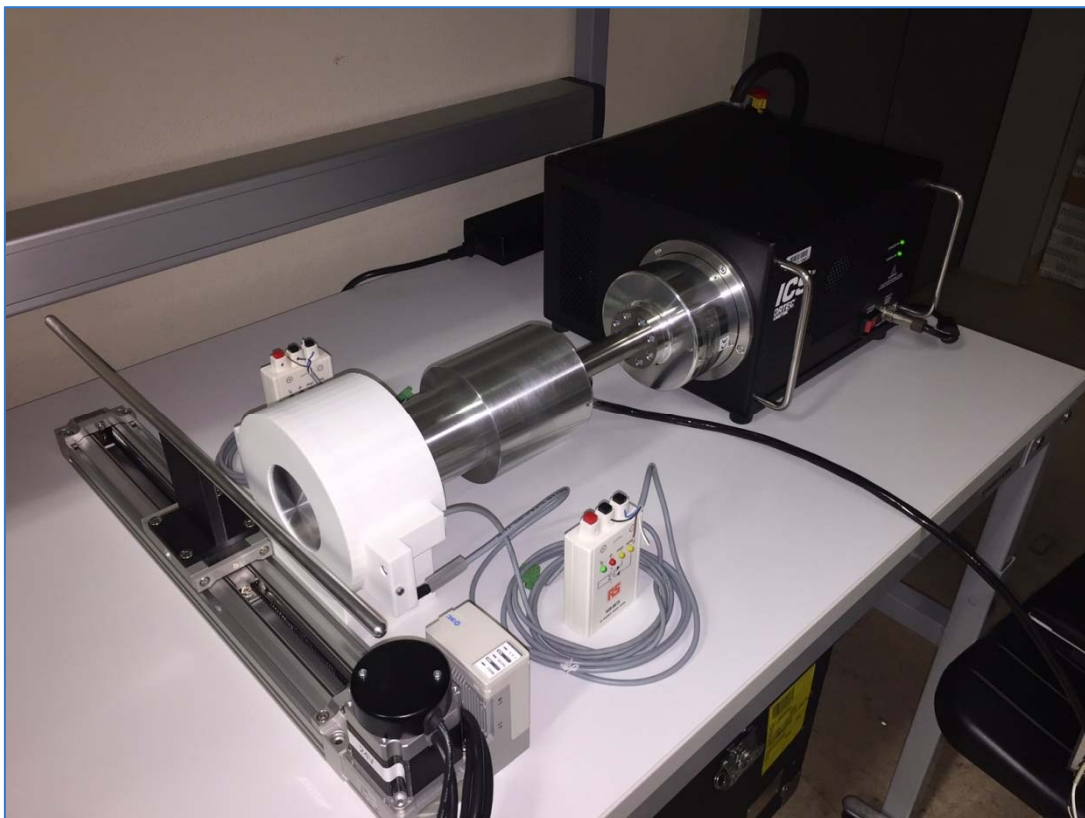
Figure 42: Testing of the fuel rod scanning system prototype
