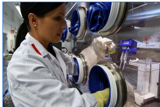
Figure 7: Pu solution weighing in glove box
