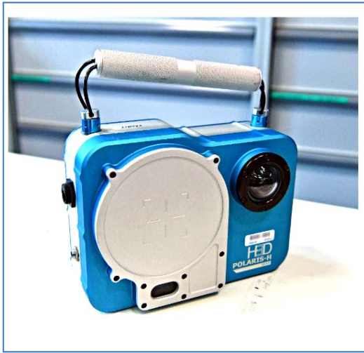
Figure 64: Gamma imaging system undergoing IAEA testing prior to authorization
