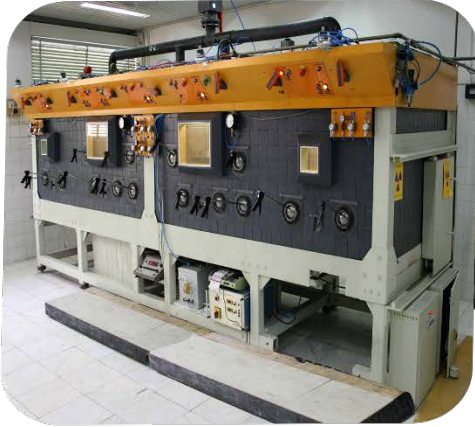
I-131 production facility
