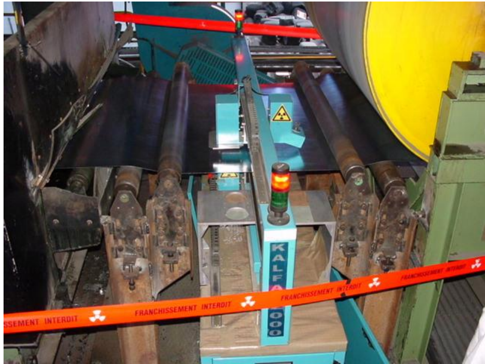
Gauge implemented on Maghreb Steel Galvanizing Line (Morocco)
