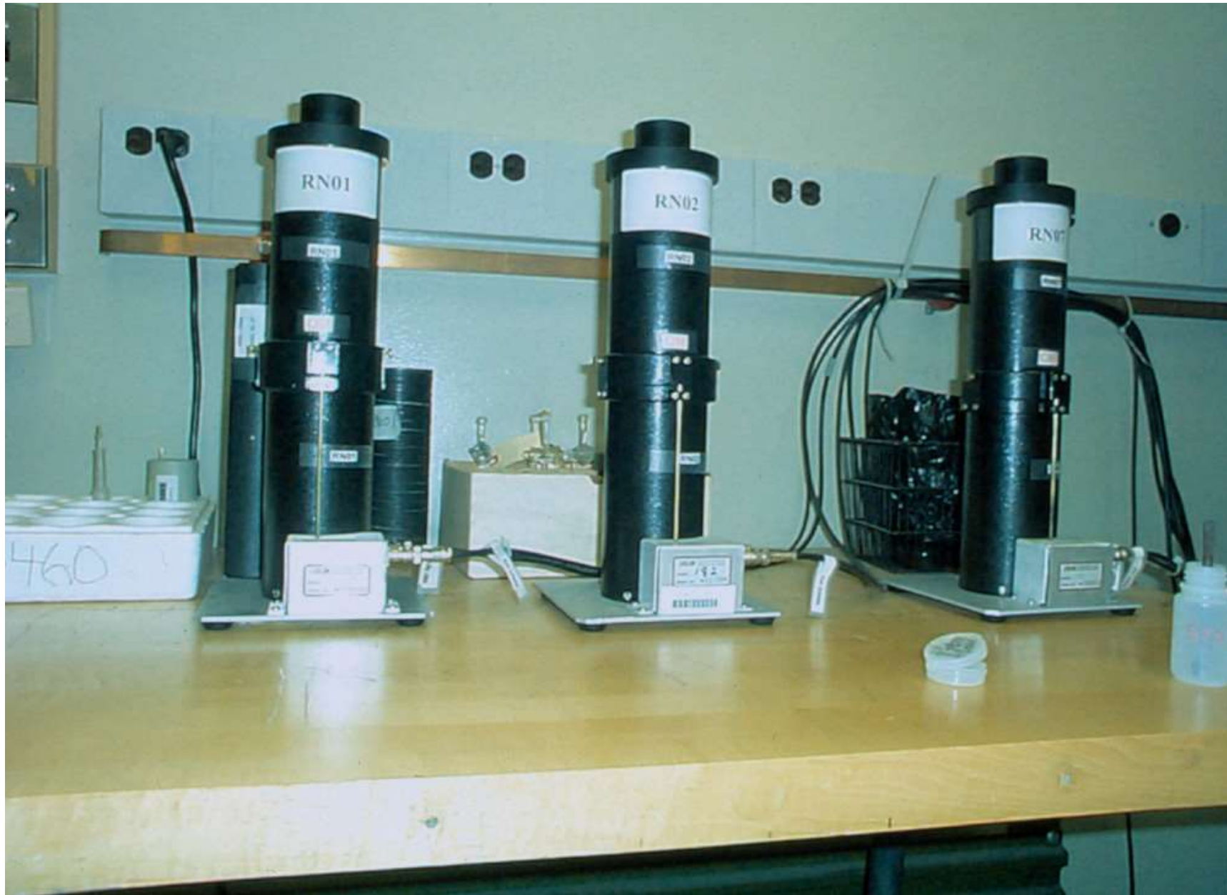
Computer controlled counters for alpha scintillation cells
