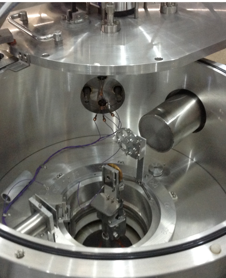
Internal view of the 17" ultra-high vacuum chamber, where a sample is installed for improved and advanced characterization of materials (photo: Yacouba Diawara/IAEA).
