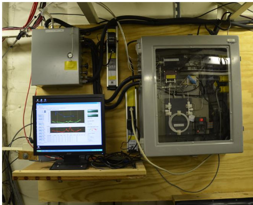
Lamont- built pCO2 Analyzer aboard the Coast Guard Cutter Healy
