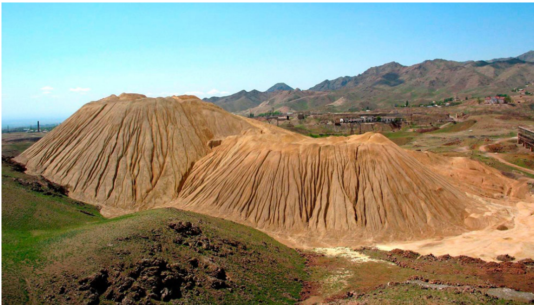
Yellow Hill - a pile of ground low grade ore remaining after leaching.
