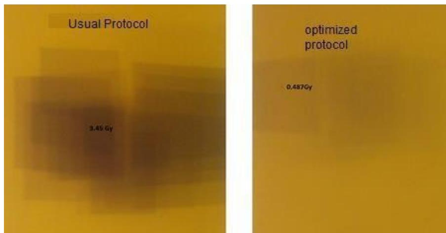
Figure 2- Patient skin dose distribution and radiation field beam variation observed on a radiochromic film used during a PAE procedures performed with the usual and optimized protocol.
