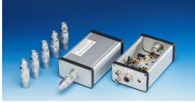
FIG. 3. Measuring set-up consisting of detectors enclosed in connectors (left) and preamplifier in aluminium housing (right).
