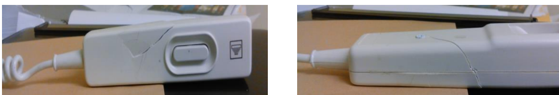
FIG. 2. Front and side view of damaged X-ray exposure switch
