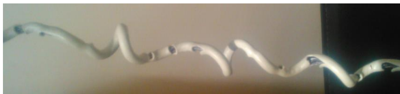
FIG. 1. Damaged intra-oral X-ray exposure cable
