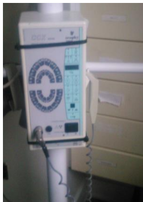
FIG. 4. Faceplate attached with cable ties
