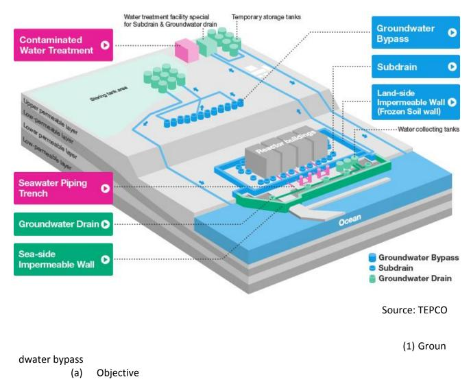
The groundwater bypass function is to isolate water from contamination by pumping it and reducing its inflow into the reactor buildings.
