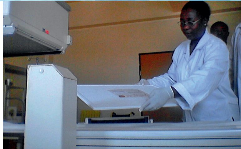
A medical physicist measures uniformity of images from a gamma camera as part of the quality assurance process.
