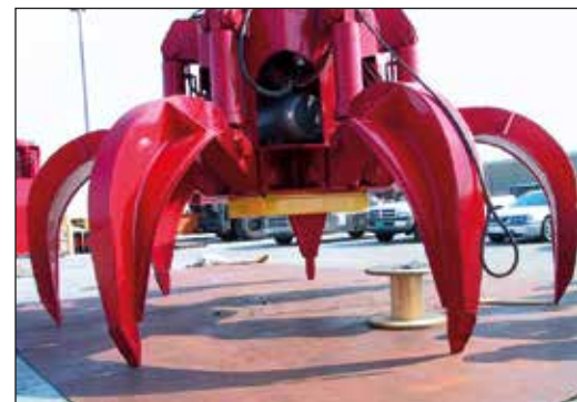
Grapple with installed radiation detector / Credit: Turner Nuclear Consulting Services, LLC.
