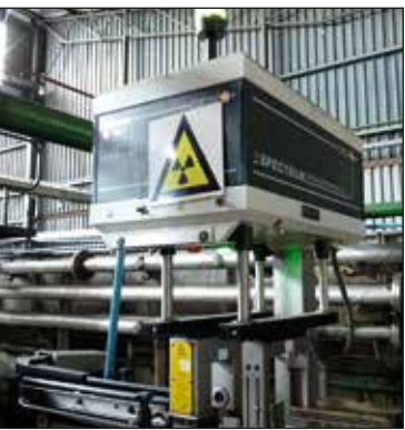
Industrial process gauge containing Am-241 / Credit: E. Reber (IAEA).
