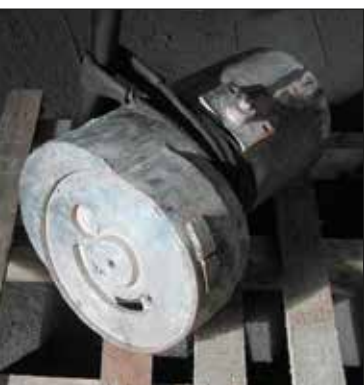
1 — Device containing 2 Curie Cs-137 source discovered in scrap metal / Credit: Turner Nuclear Consulting Services, LLC.
