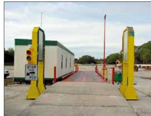
Portal monitor for detecting radioactive material in scrap metal / Credit: Turner Nuclear Consulting Services, LLC.
