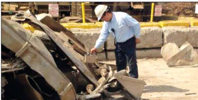
Surveying for radioactive material at metal recycling facility.
