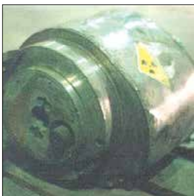
1 — Device containing 2 Curie Cs-137 source discovered in scrap metal / Credit: Turner Nuclear Consulting Services, LLC.
