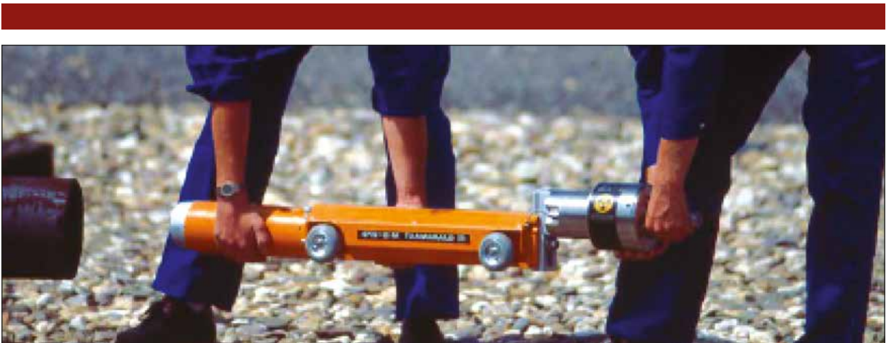
Pipeline crawler being loaded into an open pipeline / Credit: MDS Nordion.
