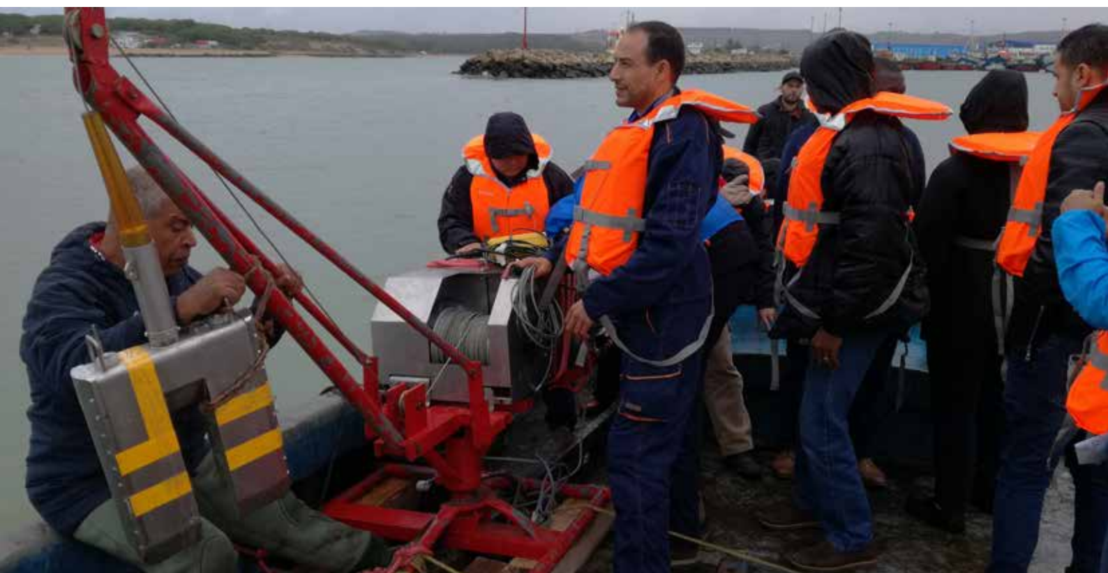
Training provided by IAEA experts on the use of a nucleonic gauge for the monitoring of sediment concentration along the access channel in Larache harbour, Morocco. (Photo: P. Brisset/IAEA)
