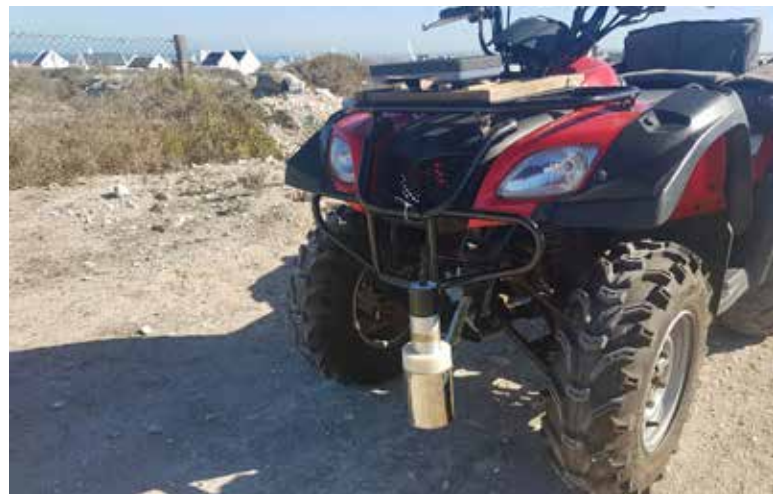
Portable gamma spectrometric detection system GISPI (Gamma in Situ Portable Device) mounted in front of a vehicle such as cars that are used to map the natural radioactivity of sediments in coastal areas. (Photo: J. Bezuidenhout/School for Science and Technology, Stellenbosch University, South Africa)
