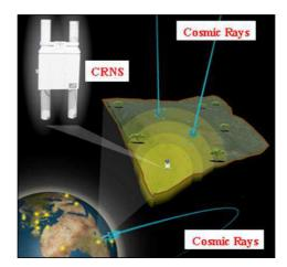
FIG. D-1. Illustration of incoming cosmic rays interacting with the atmosphere, leading to neutrons at the soil surface that can be measured by the CRNS at the landscape level. (Photo: IAEA)
