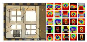
FIG. C-2. The images show an array of prototype dosimeters fabricated from synthetic device grade diamond and a montage of maps of the radiation response of the different designs measured by the IBIC technique using 5.5 MeV He+ ion irradiation. (Photos: Prof. D.Jamieson, University of Melbourne; Dr J.Davis, University of Wollongong; and Dr D.Prokopovich, ANSTO)
