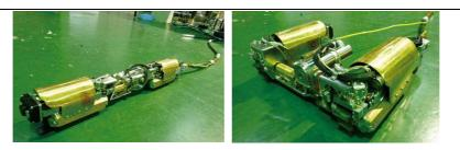
FIG. A-8. A shape-changing robot used to inspect the interior of the PCV of Unit 1 (Photos: International Research Institute for Nuclear Decommissioning, Japan).
