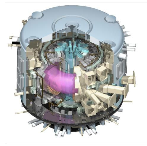
The ITER Tokamak will be nearly 30 metres tall, and weigh 23,000 tonnes. The very small man dressed in blue (bottom left) gives some idea of the machine's scale. The ITER Tokamak is made up of an estimated one million parts.
