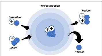
A mixture of Deuterium and Tritium — two Hydrogen isotopes — will be used to fuel future fusion power plants. Inside the reactor, Deuterium and Tritium nuclei collide and fuse, releasing Helium and neutrons. (Image: IAEA/M. Barbarino)
