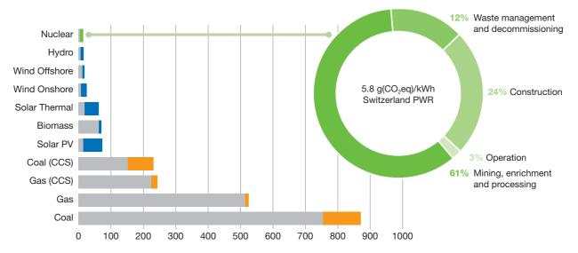
Life cycle greenhouse gas emissions per kilowatt-hour (g CO<sub>2</sub>-equivalent/kW-h)
