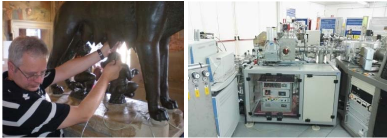
FIG. C-2. Sampling of the famous bronze Capitoline wolf at the Centre for Dating and Diagnostics, University of Salento, Lecce, Italy (left). The bronze statue had been considered to be Etruscan work from around 500 BC. Samples of the original casting cores were taken, organic residues were selected by optical microscopy, and radiocarbon dating at the accelerator end station (right) gave the final answer: the statue was made some time between 1100–1200 AD and is thus about 16 centuries younger than was thought.
