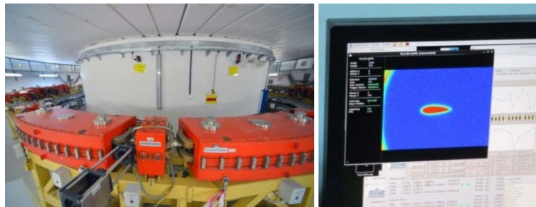
FIG. C-3. The inner storage ring of SESAME, with deflection and focusing magnets through which the electron beams circulate as they are accelerated (left). The first beam delivered, as visualized by the data acquisition system in the control room of SESAME. (Photos: IAEA)
