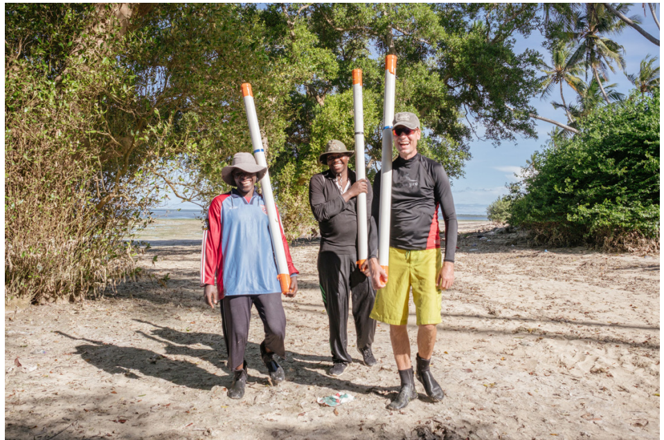
FIG. H-3. Sediment cores collected off Zanzibar, United Republic of Tanzania, to assess inventories and burial rates of organic carbon as a measure of carbon sequestration potential. (Photo: Gloria Salgado, Edith Cowan University, Perth, Australia)
