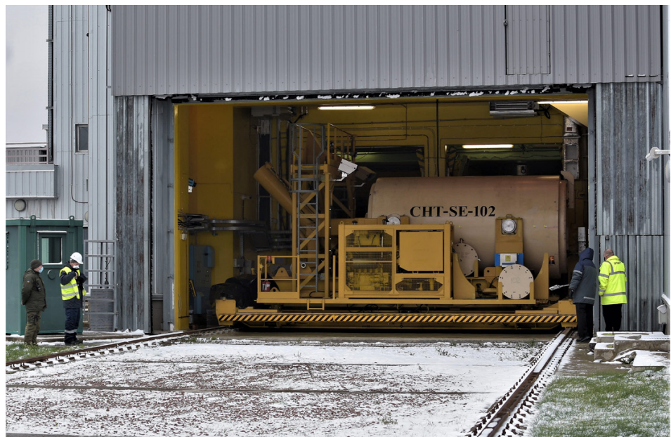
FIG. C-1. The first double-wall shielded canister filled with 93 spent fuel assemblies is leaving the Spent Fuel Processing Facility to be placed for the one-hundred-year storages. (Photo: State Specialized Enterprise Chernobyl NPP)
