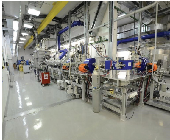
FIG. D-4. The superconducting high-power (200 kW) linear proton/deuteron accelerator (left), combined with innovative liquid lithium target technology for neutron production (right). (Image: Dan Berkowitz, Soreq Nuclear Research Center, Israel)
