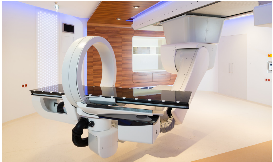
FIG. F-1. Ion beam therapy planning and implementation is one of the areas in which microdosimetry could provide a valuable contribution. The figure shows an irradiation room of MedAustron ion beam therapy centre in Wiener Neustadt, Austria, where tumour patients are treated with proton and carbon ion beams. The ceiling-mounted robotic arm holds the patient couch and the X-ray imaging ring is used for patient alignment. (Source: MedAustron, Austria. Author: Kästenbauer/Ettl.)
